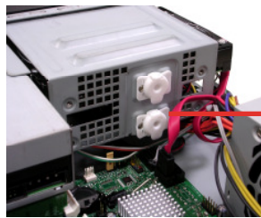
Screwless HDD, ODD assembly
