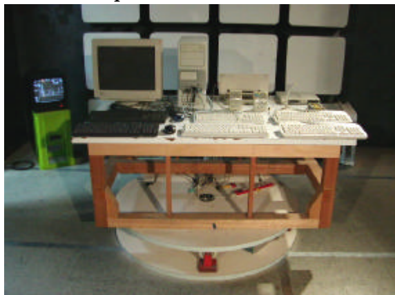
Figure 4.1.1. Generic Test set up for the Yeong Yang YY-55XX Personal Computer chassis
