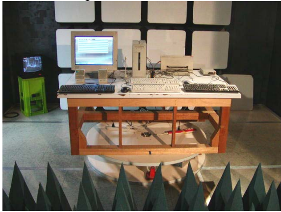
Figure 4.1.1. Generic Test set up for the Yeong Yang YY-A2XX Personal Computer chassis
