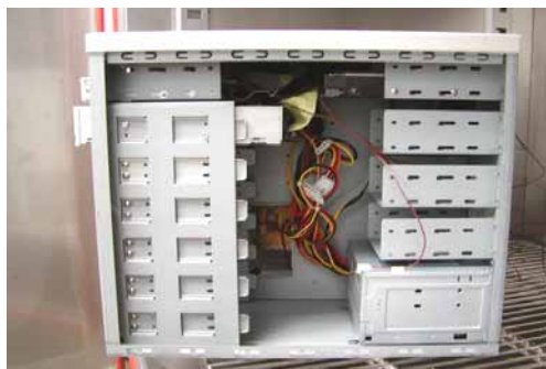
The view of system setup (HDD, CDROM, FDD, POWER).
