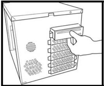
To install 3.5" HDD in the 5.25" drive bay, the metal shield could be screwed in the front end for better EMI result.
