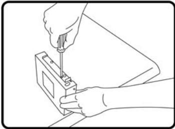
Take the metal slides out from 5.25" device frame, and ensure the metal slides should be fitted with device in position.
