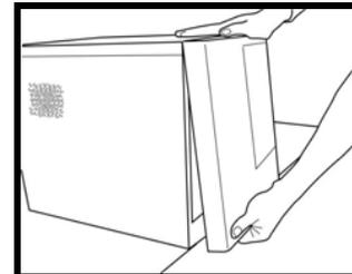
To assembly the front panel with plugging two hooks of the bottom of front panel, into the chassis body and snaps the springs of front panel in.
