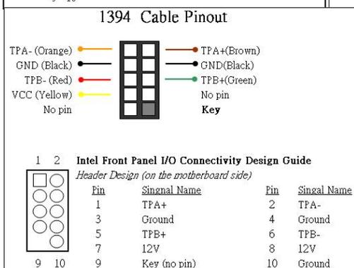
Before connecting the cables, please check pin arrangement information on the motherboard manual.
