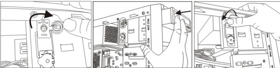
**Please make sure the front panel has been on the chassis.** The chassis designed with quick fasteners for fixing 5.25 devices.
