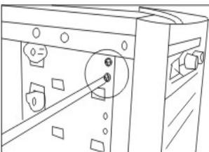
Open the fastener as marked direction. Insert the 5.25" device into the 5.25" drive bay until in correct position (hole to hole). Depress the fastener tightly.
