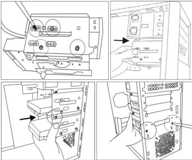
Insert the 3.5" cage with devices into the chassis, make sure the cage on rail and push towards front. Screw on the cage.
