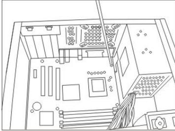
To check the mounting hole of the mainboard, screw on the optional standoffs into chassis. To install the I/O shield provided with mainboard, insert it from inside of chassis towards outside.
