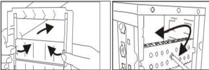
2.1. When user wants to install more 5.25"/3.5" devices – must remove the plastic dummy covers from the front panel, and the EMI shielding metal covers from the front of chassis as arrows shown. The removed EMI shielding covers could be re-used by screws.
