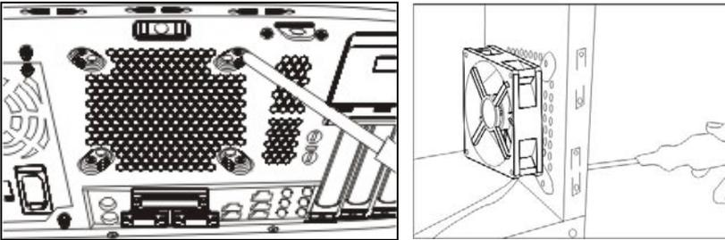
9.1. The chassis could be installed 8cm or 9cm cooling fan in the rear end of chassis.
