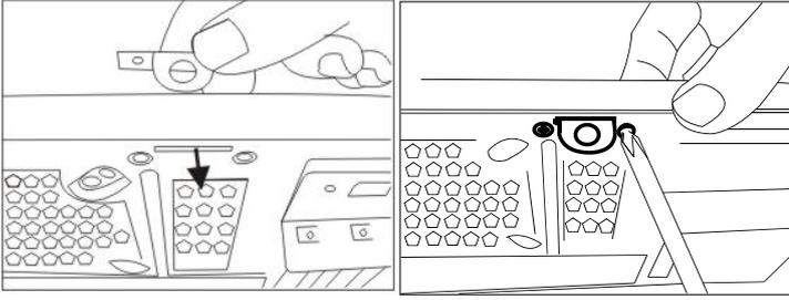
8.1. For the optional Padlock: find the bracket and flat screws (2pcs) in the accessory bag, screw on the bracket in the rear end of chassis.
