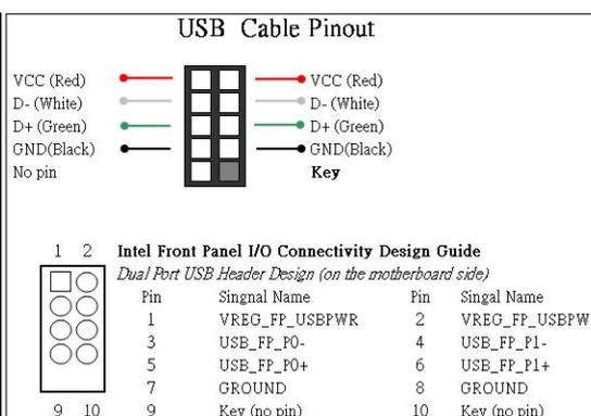
The pin out of USB2.0, AUDIO, IEEE1394 header provided by chassis is compliant with FPIO spec of [www.formfactors.org](http://www.formfactors.org)
