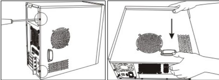
Release screws on the back of chassis.
