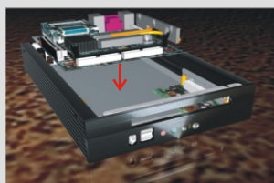
INSTALL AND FIX MOTHERBOARD
