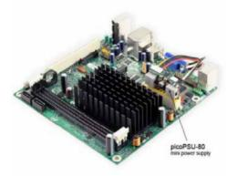
2) Connect a 12 VDC power adapter (or any 12V source) to the DC-to-DC connector, center pin / white wire is positive (+).
